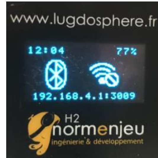
Barred WiFi logo : The dropper does not have access to the internet (hotspot or box...)
