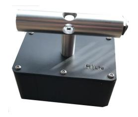
Headform H1 Lite with accelerometer
